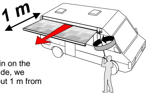
**(EN)** In order to avoid unnecessary strain on the awning as well as on the vehicle side, we suggest to take out the legs at about 1 m from the opening.
